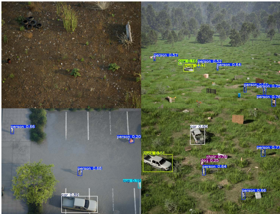
Figure 6. Color images with YOLOv12-X declarations overlaid.
